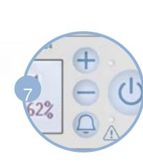
Set the flow setting to the flow rate prescribed by your clinical professional. The flow setting can be changed by pressing the circular flow setting buttons that are marked with "+" and "-" symbols. Position the nasal cannula on your face and breathe normally through your nose.
